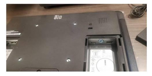
The older 1002L version doesn't have USB-C port and on the right side has only the HDMI port and micro-VGA
