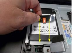
d. Remove HDD/SSD from slot and replace with compatible drive.
