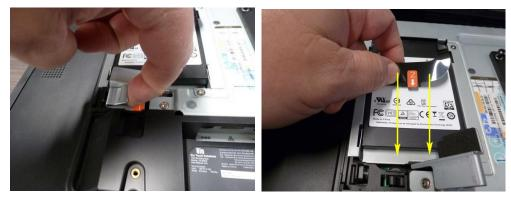
d. Remove HDD/SSD from slot and replace with compatible drive.
