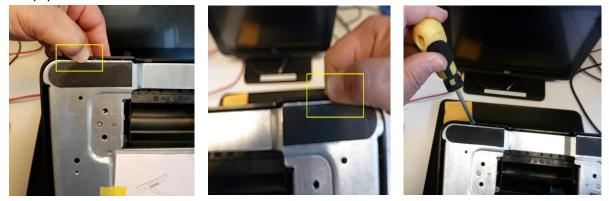
3. Support the stand cover with your hand and do not allow it to drop. Carefully slide the stand cover off making sure not to apply any downward pressure which might break off the plastic retaining tabs.
