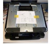
2. Use fingers to gently lift upward on corner of plastic stand cover to release the retaining clips (both left and right side). If unable to remove with fingers, use a flat blade screwdriver to gently pry outward in the location shown below until the stand cover releases.
