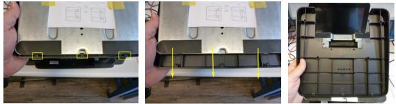
4. Reassemble in the reverse order of above, pay attention to the plastic retaining tabs and not allow them to get broken during re-assembly.
