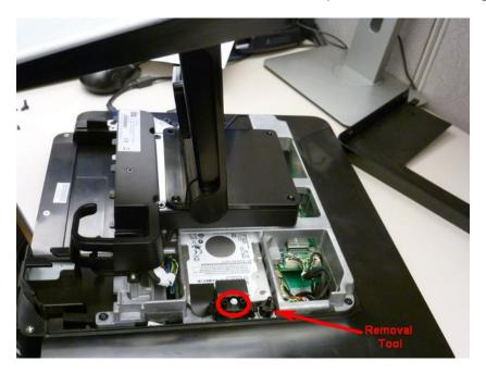
4. **To add or replace RAM:** Using fingers, or a small Philipp's screwdriver, remove thumb screw that holds the RAM cover in place and remove the RAM cover by pulling upwards.
