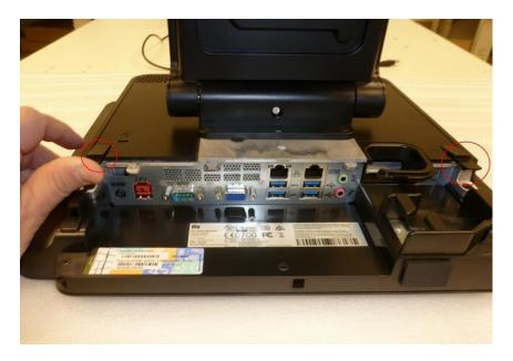
3. **To add or replace HDD:** Using the Removal Tool, unscrew the HDD retaining screw, remove retainer, slide HDD into available slot, replace retainer and tighten screw with removal tool.
