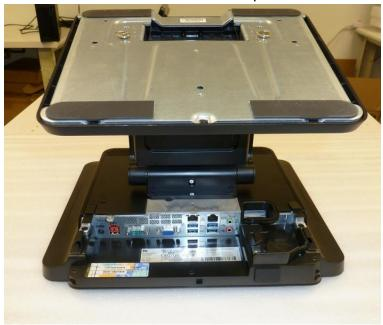
2. Using fingers pull up on the two tabs on the bottom of the back cover and push up and forward to remove the cover.
