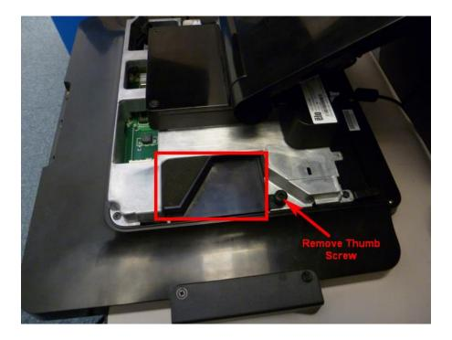
5. Once the RAM cover is removed, replace or add RAM to available RAM slots. Then place RAM cover back on and tighten with thumb screw.
