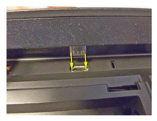
4. Be certain not to misalign the connection or it may cause the internal micro-USB connector to become bent or recessed making it unusable.
