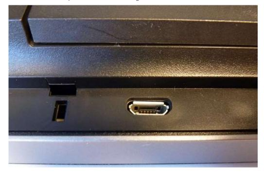
3. Carefully align the male micro-USB from the peripheral with the female micro-USB port on the edge of the monitor and gently push the peripheral into place.
