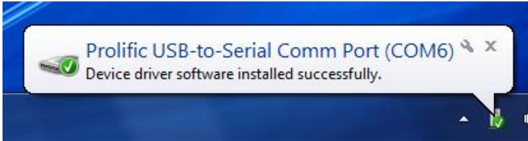
11. After Windows completes installation you can then go into the Windows Device Manager and see the new entry. In the example below it created COM6. This will be the comport that the VFD communicates through.
