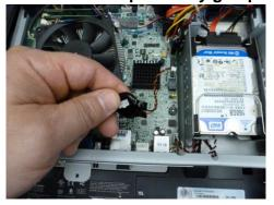
4. The BIOS battery is a CR2032 with leads. This is a very common battery which can be sourced from many places on the web such as this one: <a href="http://tinyurl.com/zvjakq7">http://tinyurl.com/zvjakq7</a>
