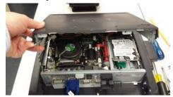
3. Remove the BIOS batter lead from the Motherboard. The BIOS battery is stuck to the back of the audio jack housing with a piece of double sided tape. Firmly grasp the battery and pull it off.
