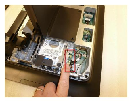
4. Using a small Philipp's screwdriver, remove the two screws that secure the Wi-Fi adapter.
