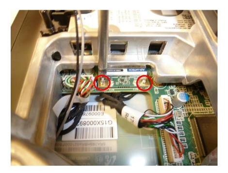
5. Once the two screws are removed the Wi-Fi adapter will lift upwards.
