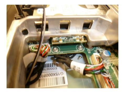
6. Using your fingers, remove the Wi-Fi adapter out of the unit.
