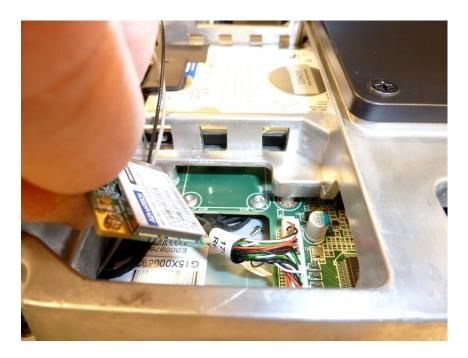
7. If you are not going to be replacing the Wi-Fi adapter, wrap the antenna connectors with electrical tape to prevent any accidental electrical shorts. If replacing the Wi-Fi adapter, slide the new adapter into the slot and reassemble in the reverse steps as disassembled.
