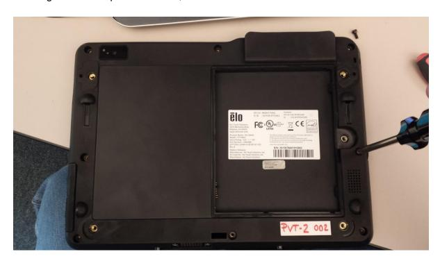
5. With your fingers, carefully pry apart the two halves of the Tablet, start at the top of the Tablet.
