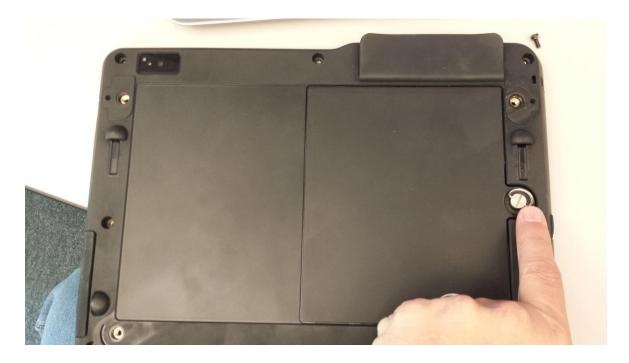
4. Using the #2 Phillips screwdriver, remove the 8 screws that secure the Tablet.
