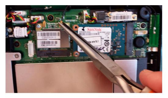
7. Using the #1 Phillips screwdriver, remove the two screws that hold the card in and remove card.
