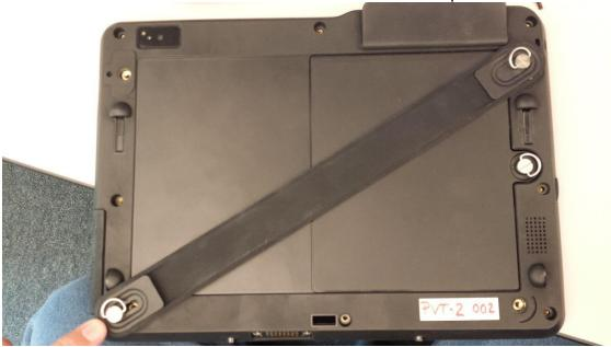
3. Remove the thumbscrew which secures the battery, and remove the battery.
