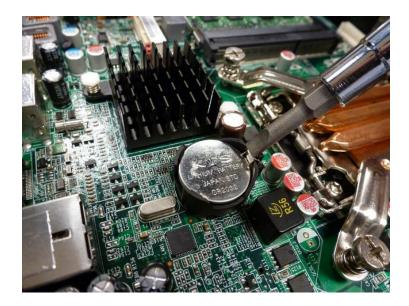
5. Battery will spring upward for removal.
