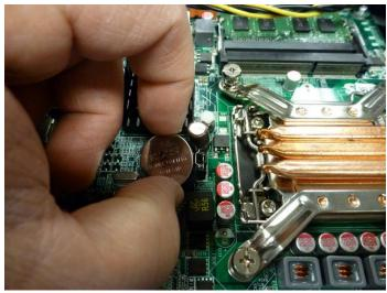
6. Place new CMOS battery into battery slot. Using finger, press downward on battery until it snaps into place.
