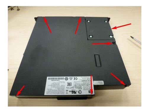
2. Using the flat blade screwdriver, remove the slotted silver slide screw from the side of the module.
