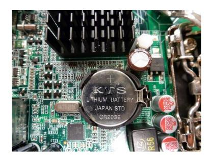
4. Using flat blade screwdriver, push spring clip to release battery.
