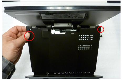
2. Using fingers or the Philipps screwdriver, remove the large black screw that holds the front metal plate.
