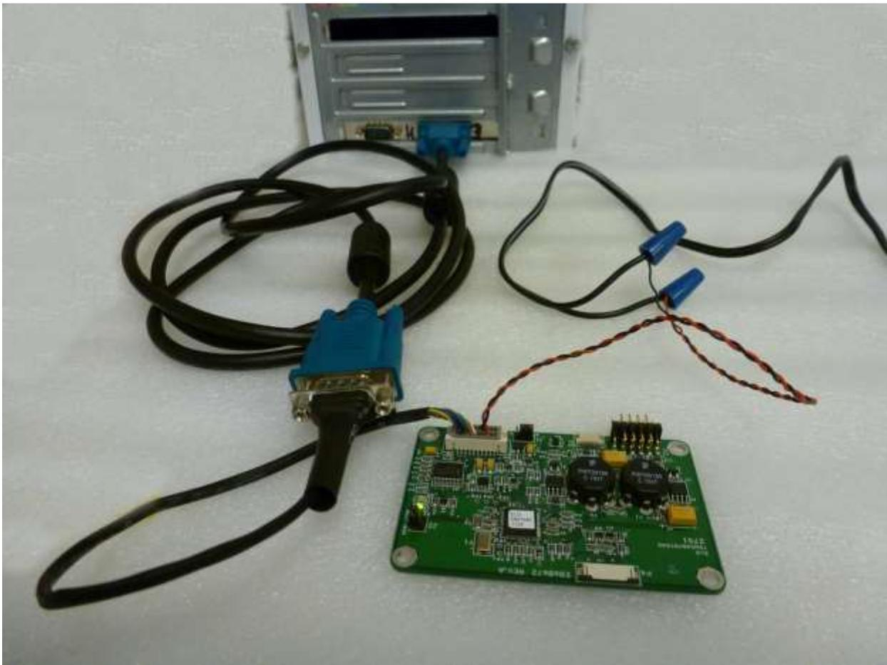
3. Connect the 2 X 20 Connector from the Elo Wiring Harness to the mating connector on the 2701 Controller. The LED's on the controller should now be blinking green.
