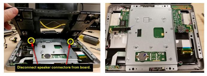
Elo Touch Solutions, Inc. | 670 N. McCarthy Blvd, Milpitas, CA 95035 | 1-800-557-1458 | <u>elotech@elotouch.com</u> ©Copyright 2019 Elo Touch Solutions, Inc. Confidential & Proprietary, Subject to NDA. 6. Use flat blade screwdriver to lift CMOS battery up out of retainer.
