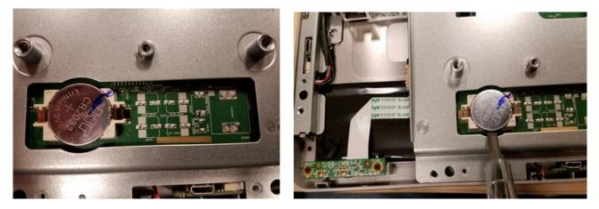
7. Replace CMOS battery with a +3V Lithium Coin type CR2032 battery.
