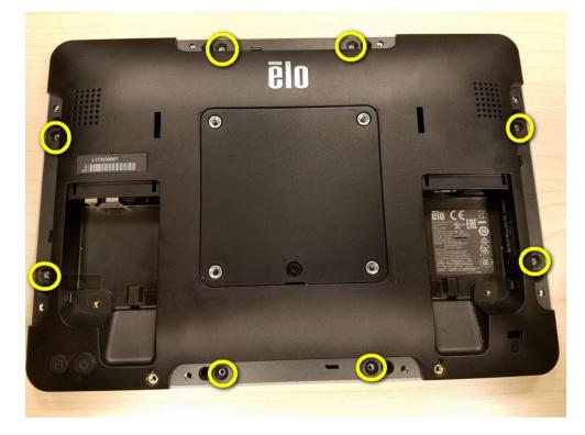
2. Remove the center cover screw and lift off center cover.
