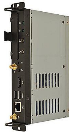
Example of OPS Digital Signage computer
