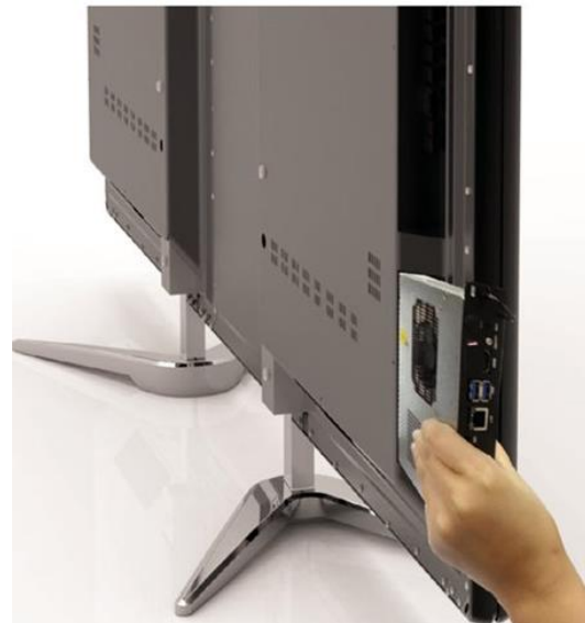
Example OPS being connected to a 3rd party IDS monitor
