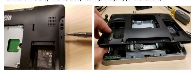
5. As you lift back cover, notice the speaker wires that are connected to the board. These must be disconnected to completely remove back cover.
