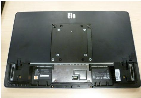
2. Using fingers pull up on the two tabs on the bottom of the back cover and push up and forward to remove the cover.
