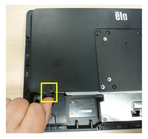
3. Remove two Philipps screws from metal plate and remove plate.
