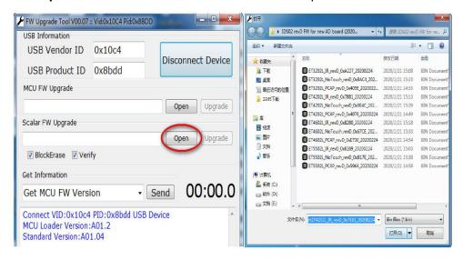
4. Click *Upgrade* to start the program. When upgrade is completed a message will appear stating: "*Scaler FW Upgrade Completed*" click on the "*OK*" button.
