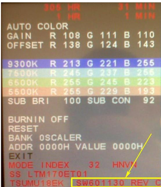
Individual functions in the Factory Menu cannot be performed without a wired OSD remote connected – with a wired OSD remote you can scroll up or down and press Select to execute Reset or Exit. To completely exit Factory mode, turn the monitor off.
