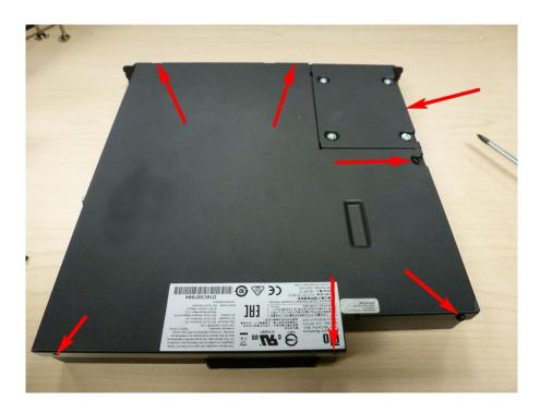
2. Using the flat blade screwdriver, remove the slotted silver slide screw from the side of the module.
