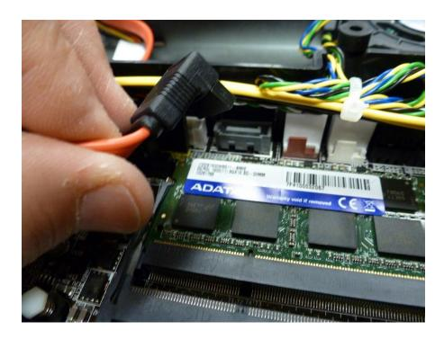
5. Push the two retaining spring tabs outward to allow RAM module to be removed.
