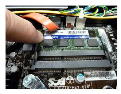
4. Disconnect the SATA connector to allow easy access to RAM module.
