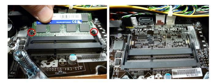
6. Replace or add extra RAM and reassemble ECM computer module by following this procedure in reverse.
