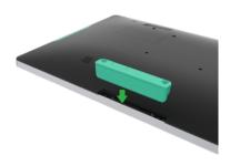
Gently insert the status light kit into the peripheral bay taking care to ensure the connector mates properly
