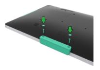
Install the 2 flat head screws included with the kit and cover the screws with the adhesive mylar covers if desired
