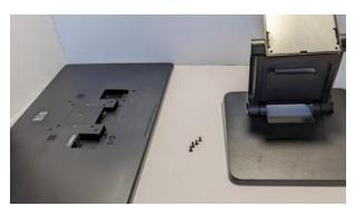
3. Place stand VESA mount over VESA mounting holes on back of I-Series, insert all 4 VESA screws and tighten with a Philipps screwdriver (stubby, small, or angled screwdriver will work)
