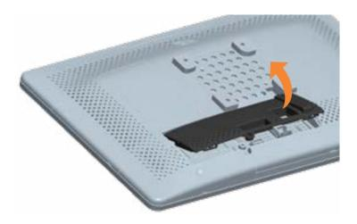
Remove and save screw and connector cover.
