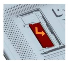
Insert the memory module into the rear slot at an angle and then press down to lock it into place. Replace DDR cover and cable cover.
