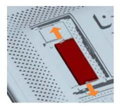
To remove existing memory modules, pull the tabs on each side out and the module will pop up.
