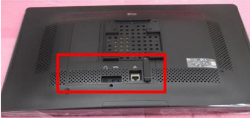
2. Plug in **USB C power adapter** and **USB thumb drive** as shown.
