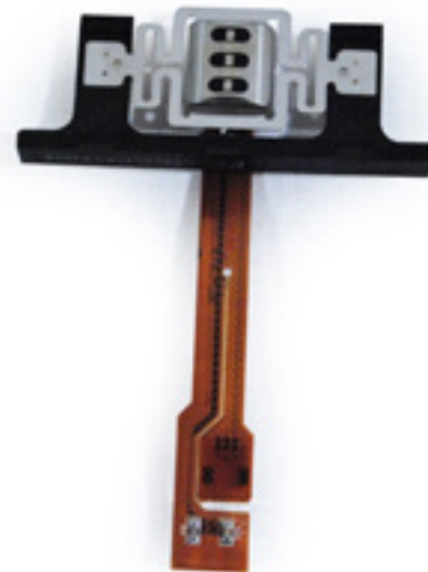
MagneSafe IntelliHead Accordion Spring U-bracket USB Connection (UART, SPI not pictured)
