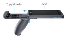
• Insert the M50 horizontally into the male USB-C on the trigger handle.
