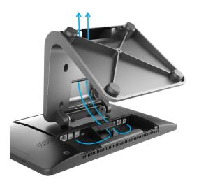
Route cables under routing clip and through stand.
